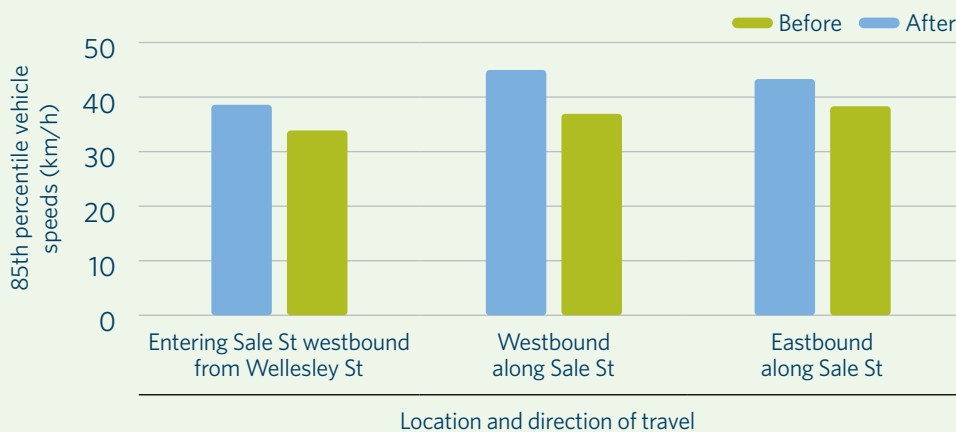
Figure 2: 85th percentile vehicle speeds on Sale Street before and after intersection improvements
