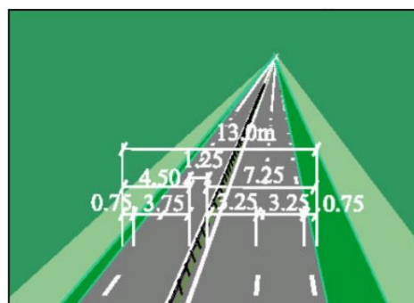
Figure 3: Drawing of 13 m 2+1 road with 1,25 m wide median and a wire rope barrier,
