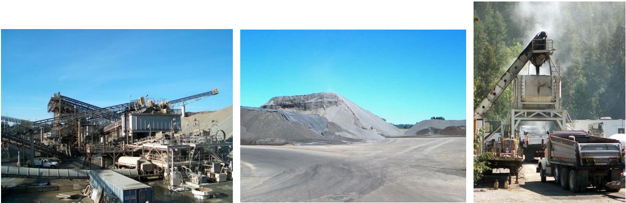
Figure 3: Aggregate production, stockpiling, and mixing
