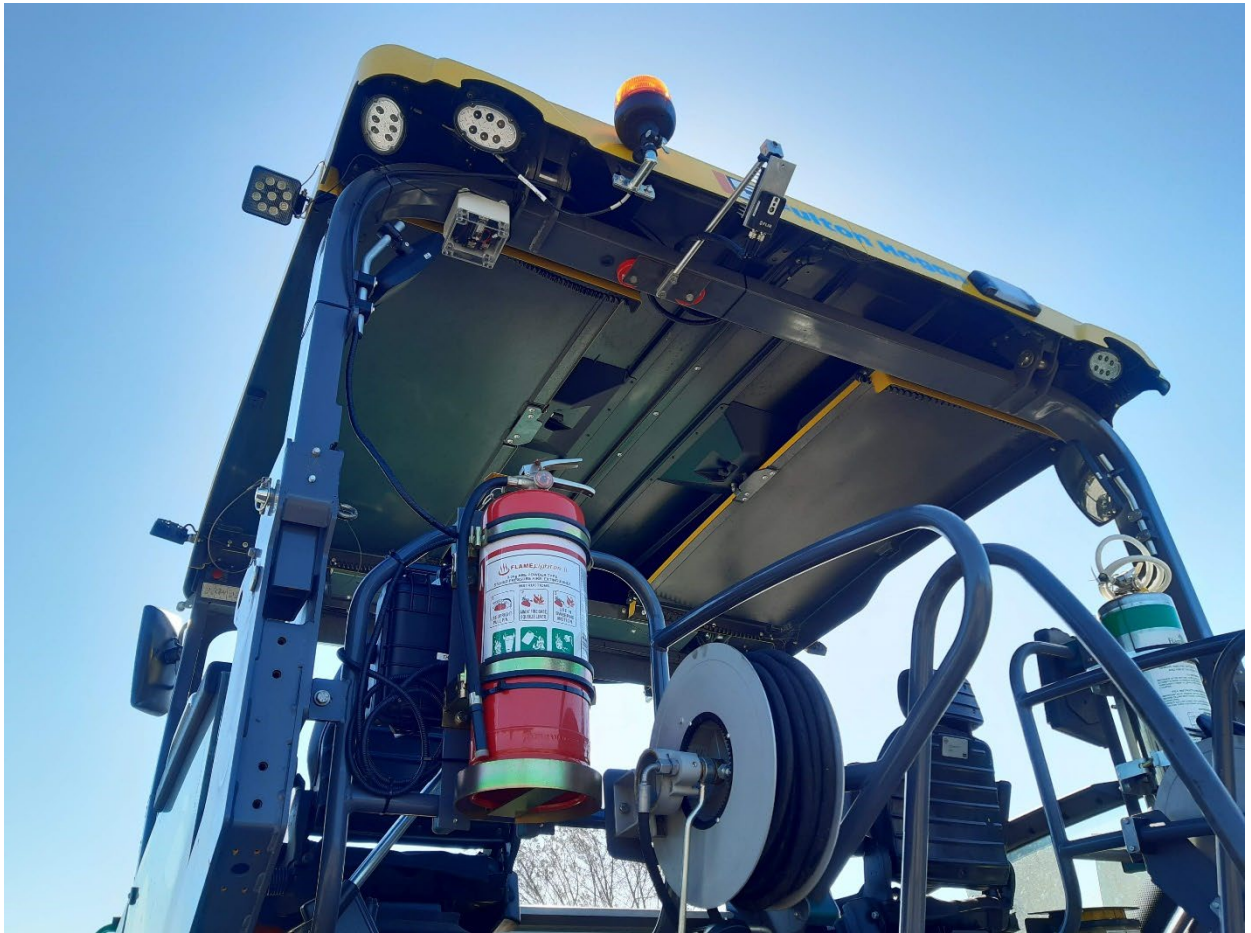
Figure 1: GPS logger and FLIR thermal imaging camera installed on paver
