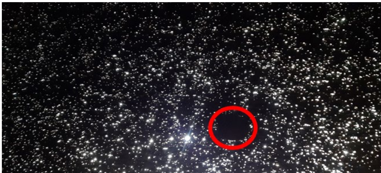
Figure 21: Aluminium disk glued to chipseal (below bitumen pre-spray)
