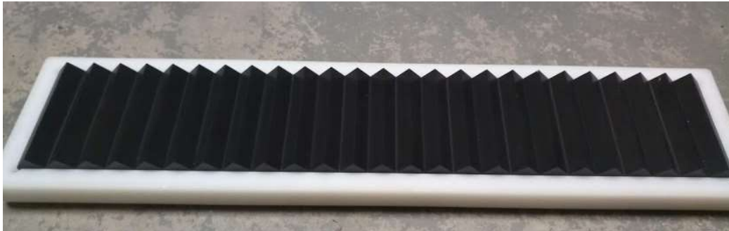
Figure 13: CAPTIF surface texture calibration plate
