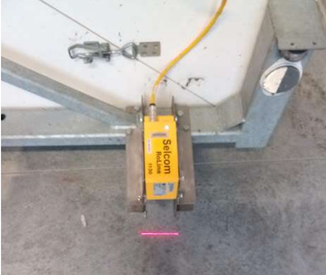
Figure 4: Laser mounted to front of CPX trailer
