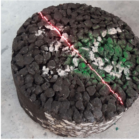
Figure 16: Core sample being measured by laser
