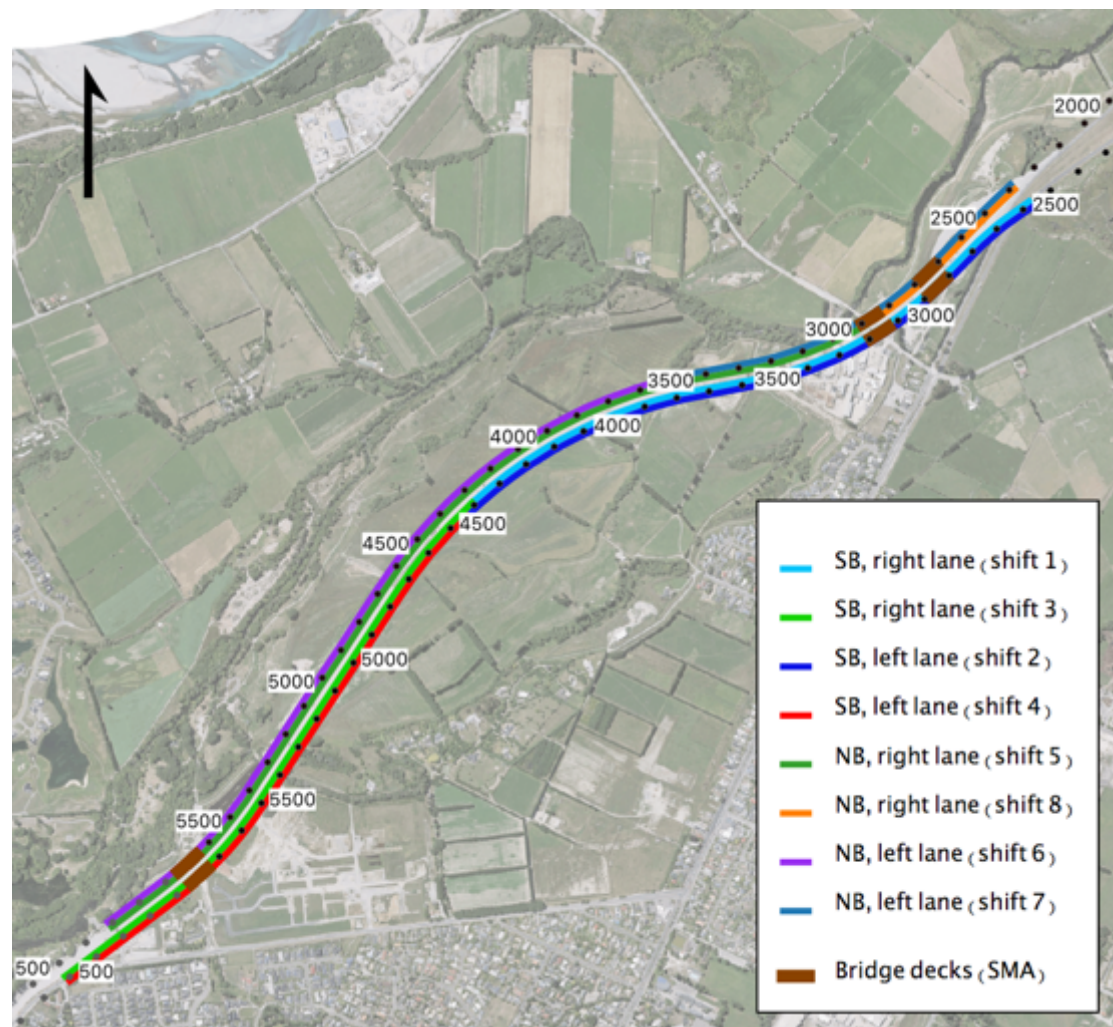
Figure 3 Extent of paving shifts. The displacement values are the Rp in metres from Rs 01S-0327 (black marks) and Rs 01S-0333 (grey marks).
