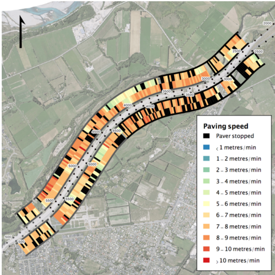
Figure 16 Paving speed and stops for WBB (20 metre segments). The construction shifts are marked as northern half (black) and southern half (grey).
