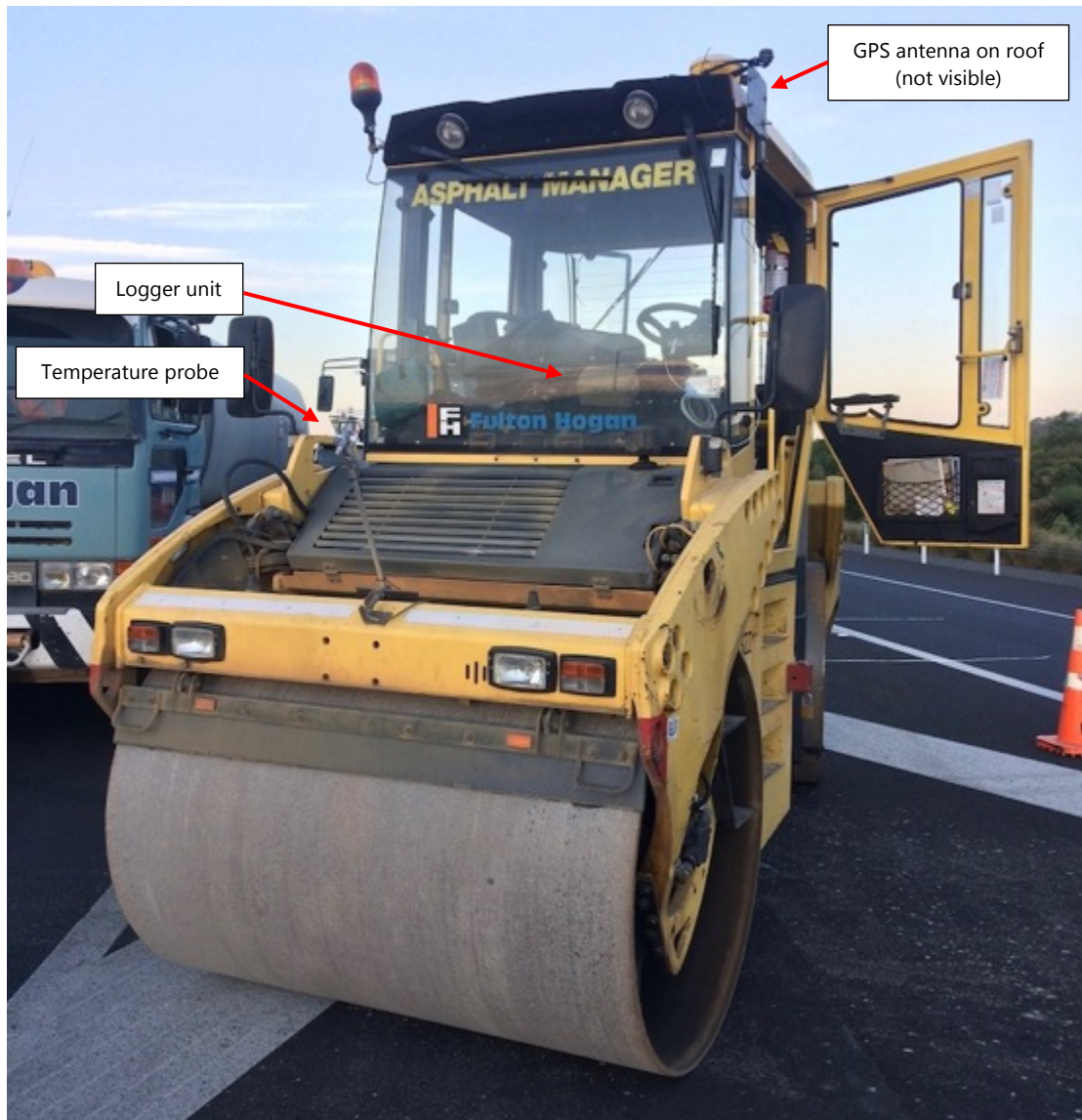
Figure 75 Temperature logger positioning on roller
