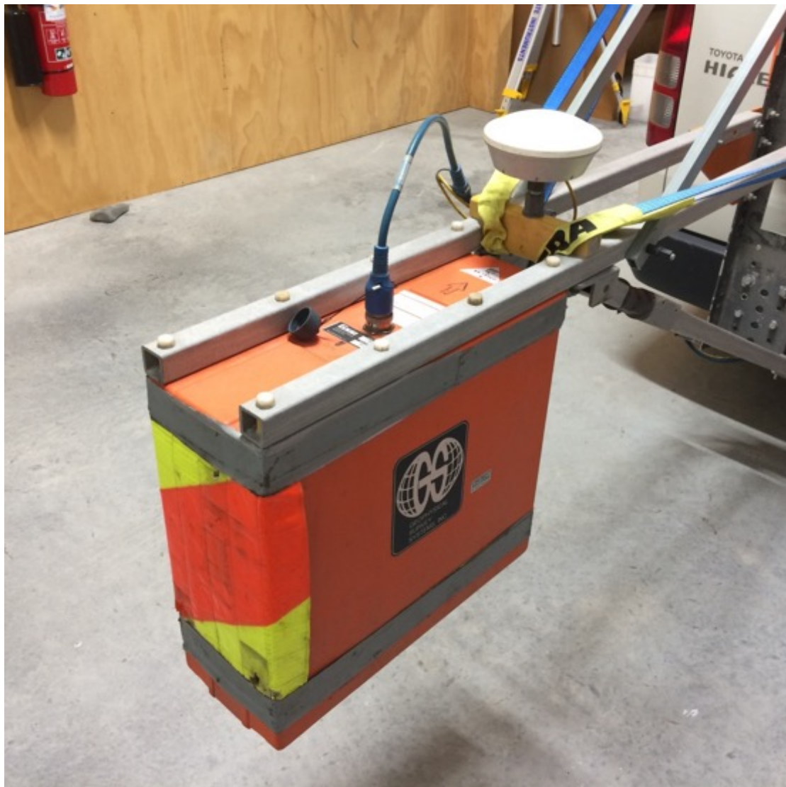
Figure 66 Fulton Hogan GSSI SIR20 GPR system with 2 GHz horn fitted to the survey vehicle.
