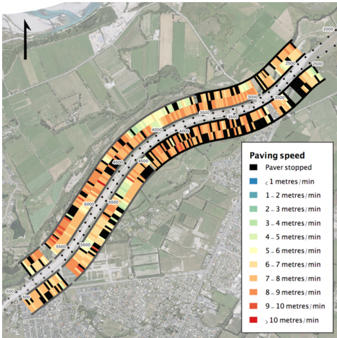
Figure 15 Paving speed and stops for WBB (20 metre segments). The construction shifts are marked as northern half (black) and southern half (grey).
