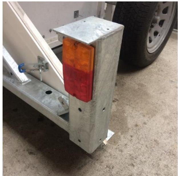
Figure 14 New LED lights attached directly to the frame, with internal cable routing
