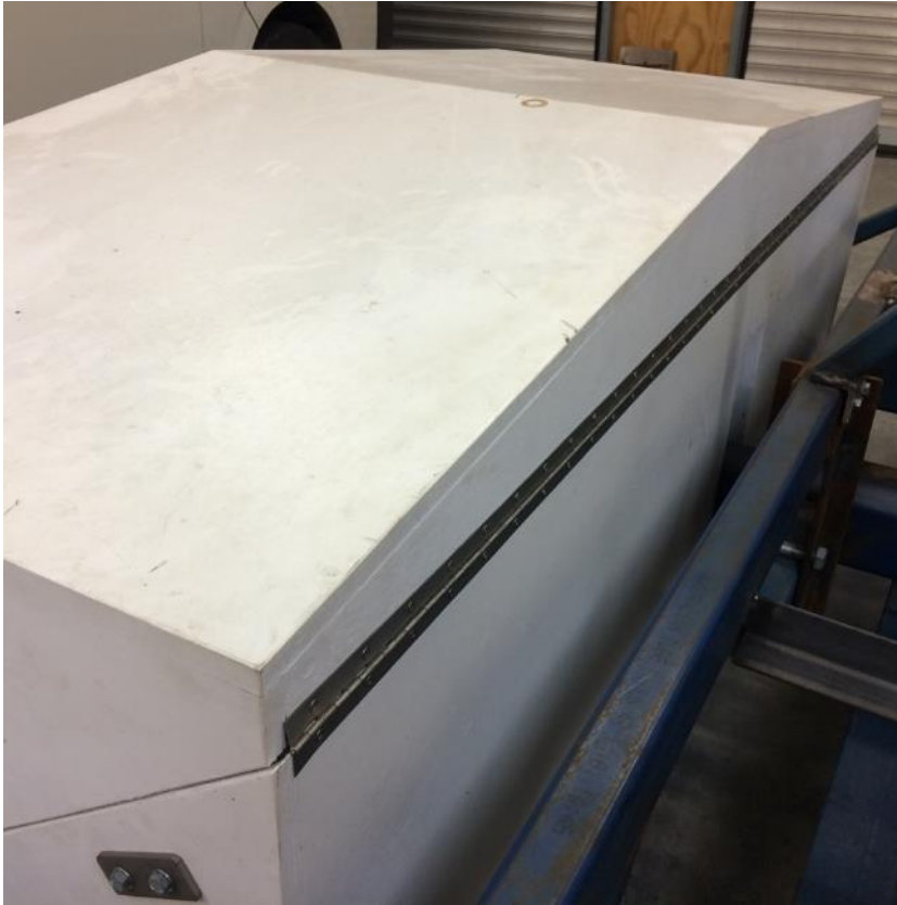
Figure 7 Wheel enclosure hinge originally under significant loads
