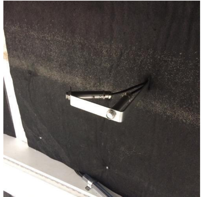
Figure 18 New IR temperature sensor located on wheel enclosure lid
