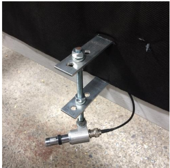
Figure 16 New microphone mounts attached directly to the wheel enclosure
