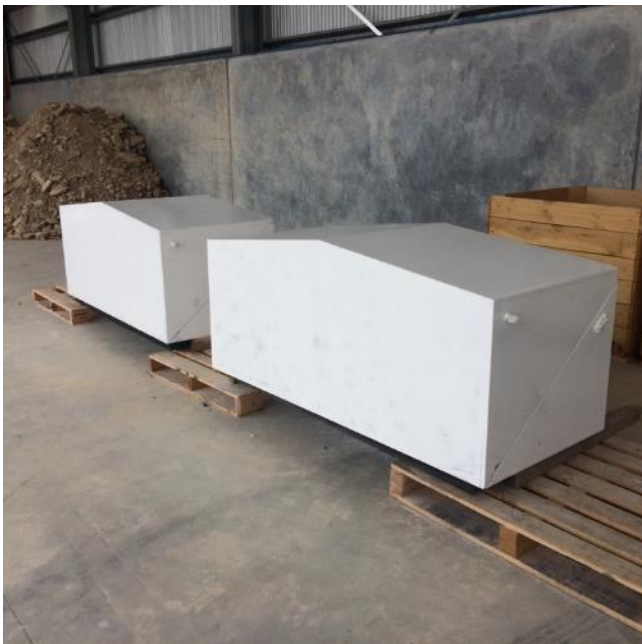
Figure 19 Wheel enclosures after first coat of paint
