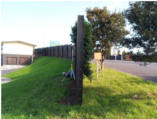
Figure 4: Microphone array and loudspeaker during sound insulation tests at Maioro Street.
