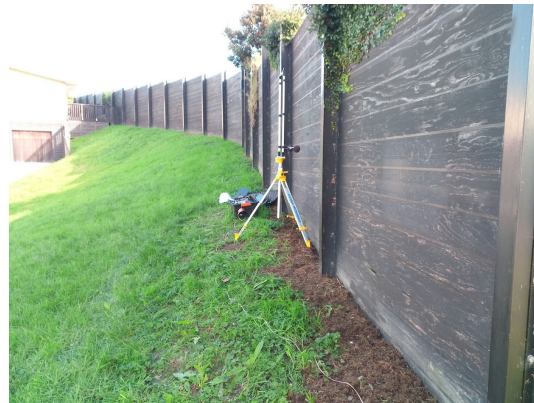
Figure 5: Microphone array during sound insulation tests at Maioro Street.
