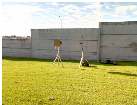
Figure 12: Microphone array and loudspeaker during free-field measurements at McCormick Green.
