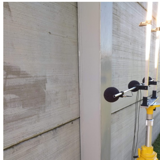
Figure 10: Microphone array during sound insulation and reflection index of posts at McCormick Green.
