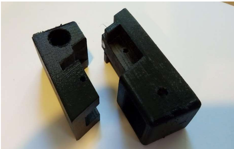
Figure 7 Microphone array – clips for shifting microphone array
