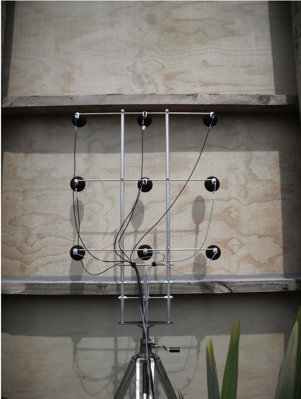
Figure F.2 Test arrangement showing the microphone array when measuring across an element
