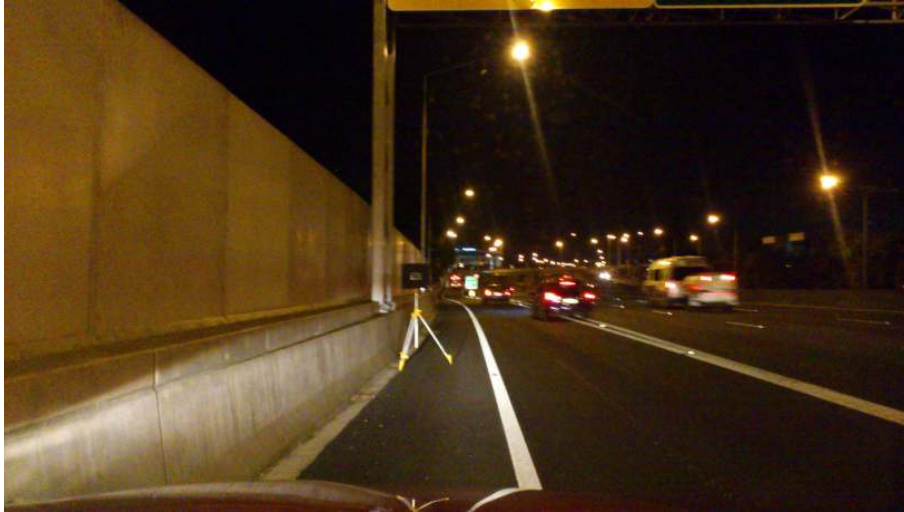
Figure G.2 Test arrangement showing the loudspeaker when measuring across an element
