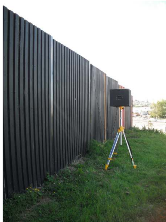
Figure D.2 Test arrangement showing the loudspeaker when measuring across a post
