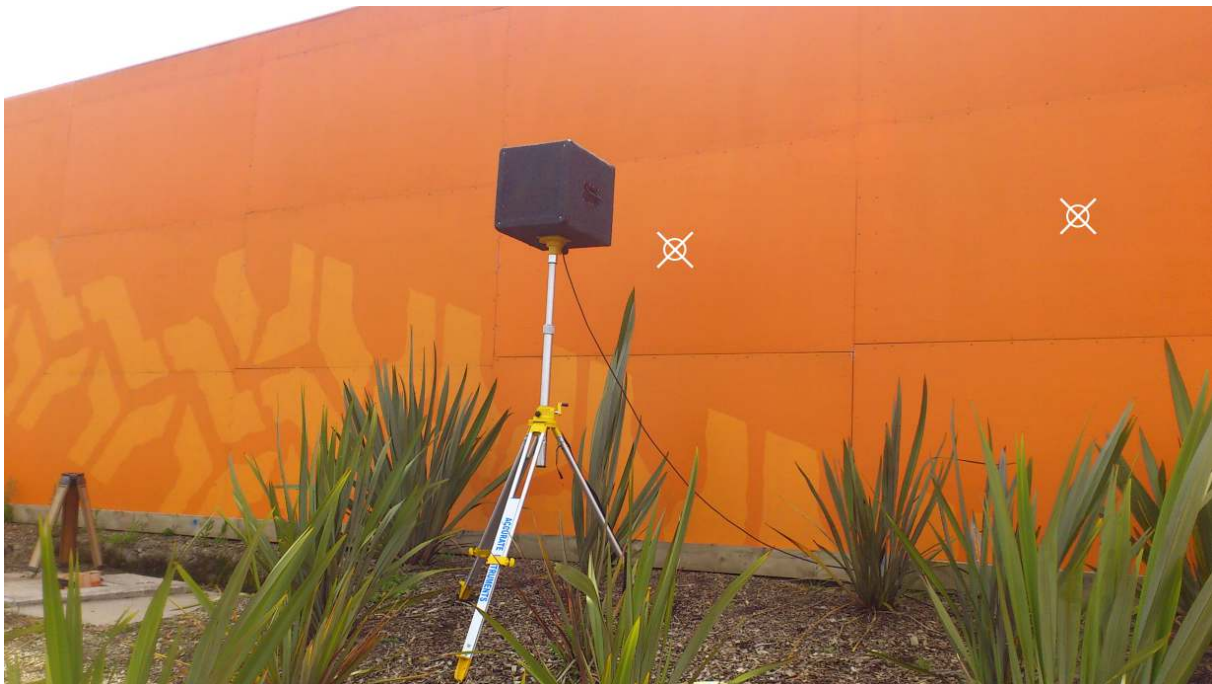
Figure F.1 Test arrangement showing the loudspeaker when measuring across an element, the crosses mark the measurement positions
