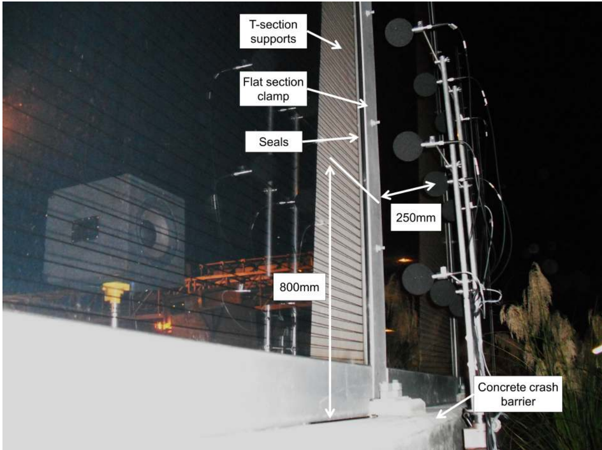
Figure B.3 Composition of the acrylic traffic noise barrier, test setup during a post measurement (position 2)
