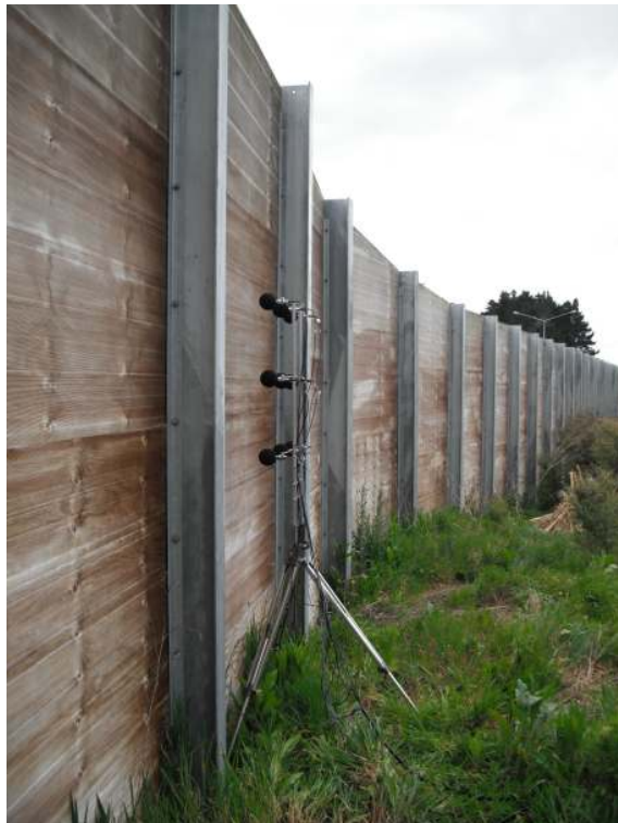
Figure C.3 Test arrangement showing the microphone array when measuring across an element
