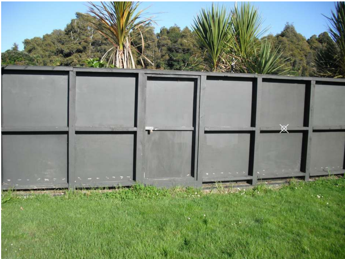
Figure I.1 Test arrangement showing the microphone array when measuring across an element, the cross marks the measurement position
