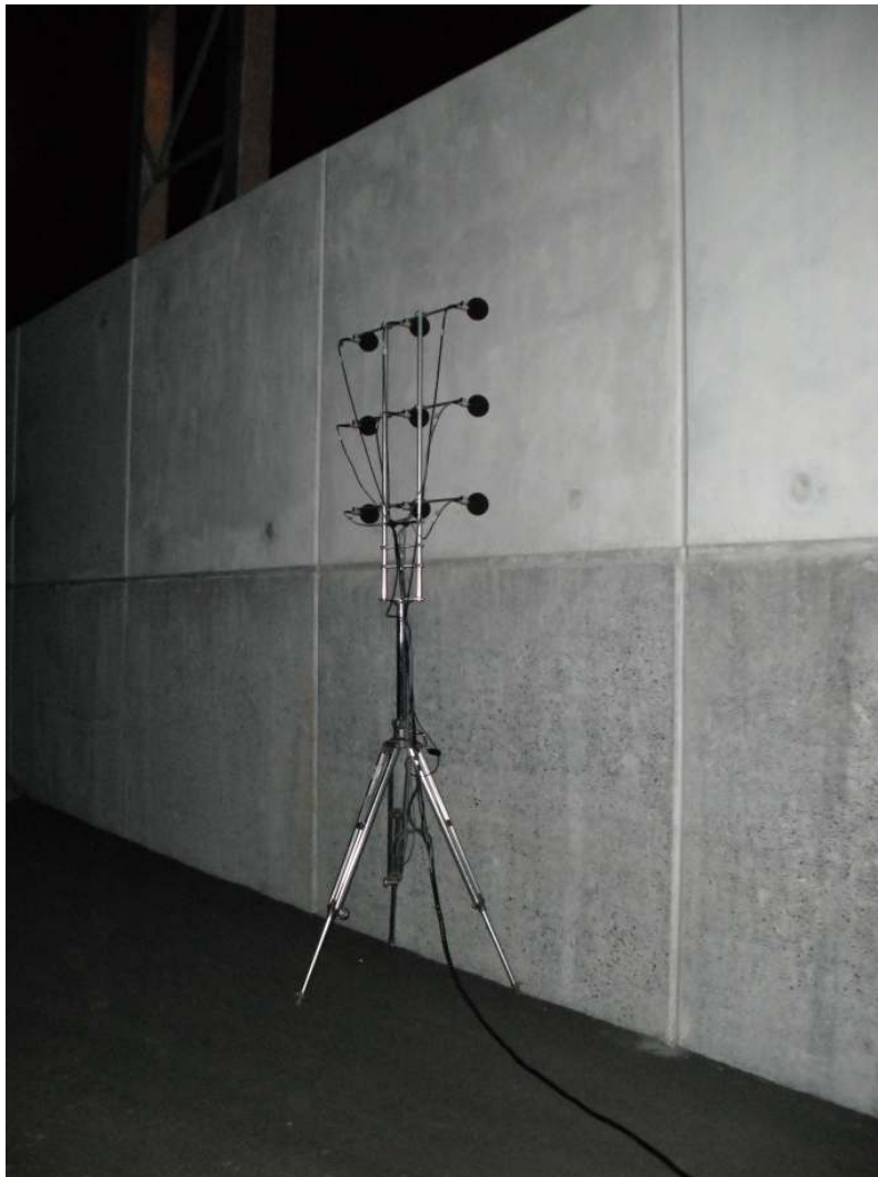
Figure G.3 Test arrangement showing the microphone array when measuring across an element
