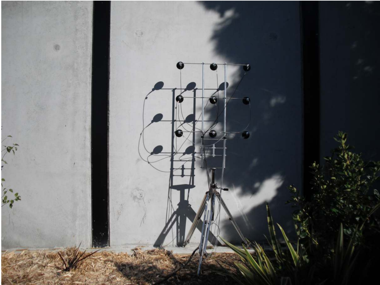
Figure E.2 Test arrangement showing the microphone array when measuring across an element
