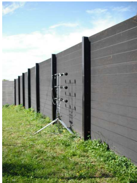
Figure D.3 Test arrangement showing the microphone array when measuring across an element
