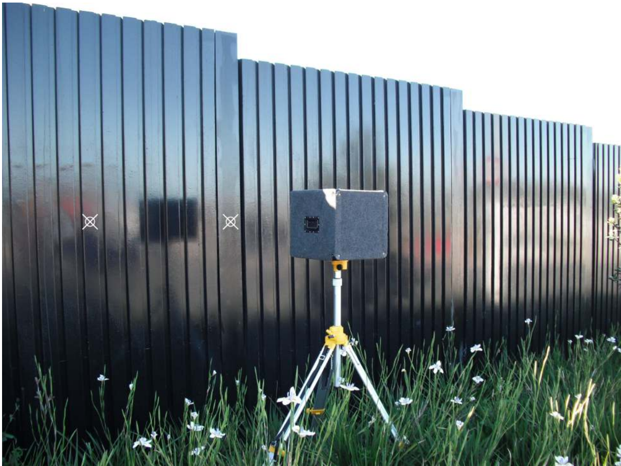
Figure E.1 Test arrangement showing the loudspeaker when measuring across a post
