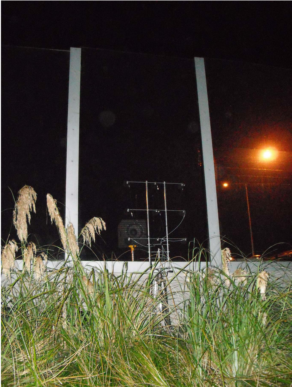
Figure B.2 Test arrangement showing the microphone array when measuring across an element (position 3)
