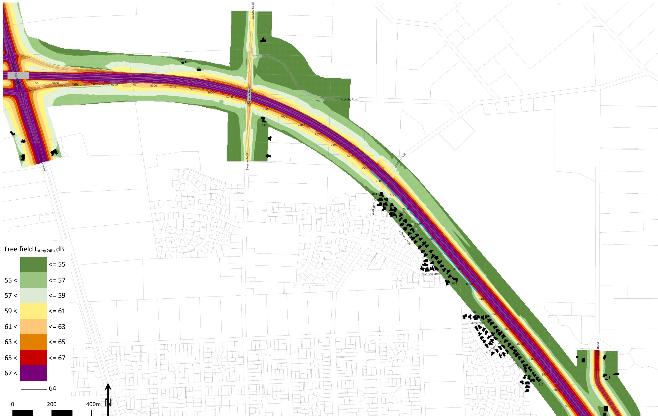
Figure D- 3 Noise contour diagrams for the BPO: Victoria Road (SH 1B) to Thornton Road (chainage 5600 to 9100)
