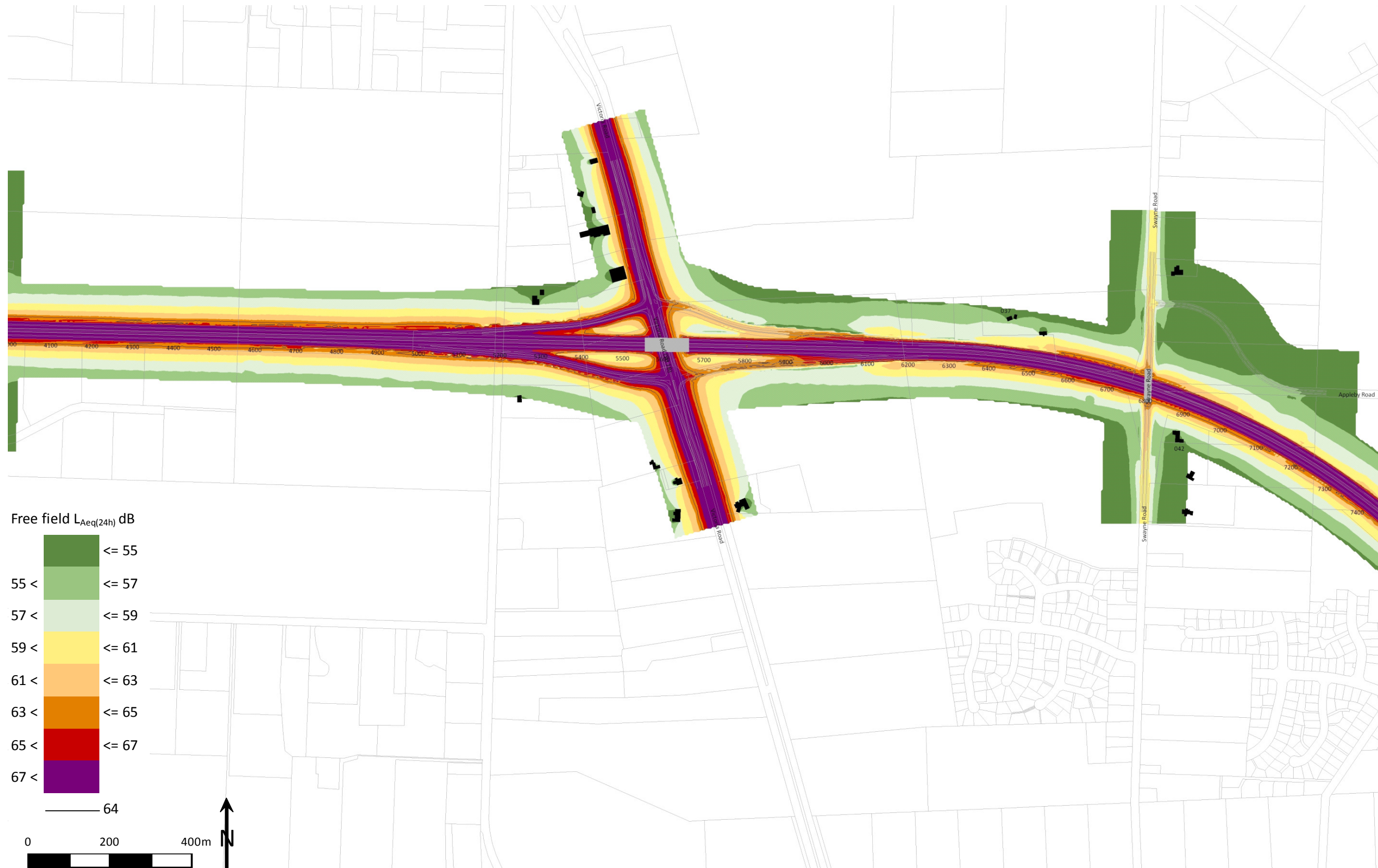
Figure D- 2 Noise contour diagrams for the BPO: Peake Road to Swayne Road (chainage 4000 to 7400)
