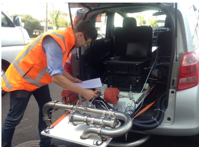
FIGURE 5.1 The PEMS equipment being installed in a test vehicle
