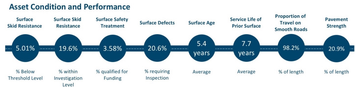
Figure 17 – Asset condition and performance summary
