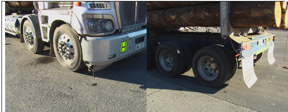
Figure 5. Sprayer units fitted to the test vehicle.
