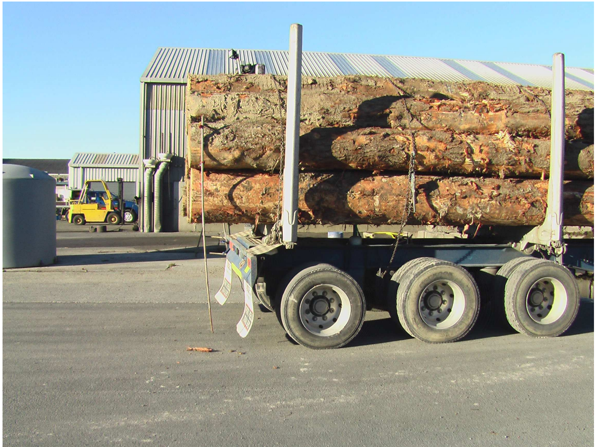
Figure 2. Load overhang for test vehicle.
