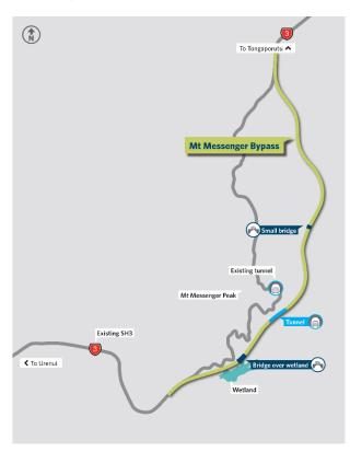
The project re-aligns SH3 in North Taranaki between Uriti and Ahititi, and consists of 5.2km of new road, two bridges and a 230m tunnel. The project replaces the existing road, which is windy, steep and prone to slips. SH3 is a high freight route and any closure at Mt Messenger causes significant delays with the main detour adding approximately four hours of travel.
