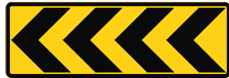
PW-69 ROUNDABOUT CHEVRON BOARD
