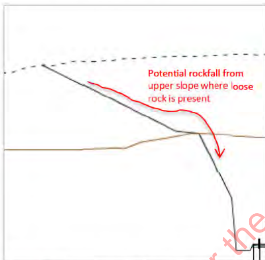
Figure 3: Potential Rockfall Risk
