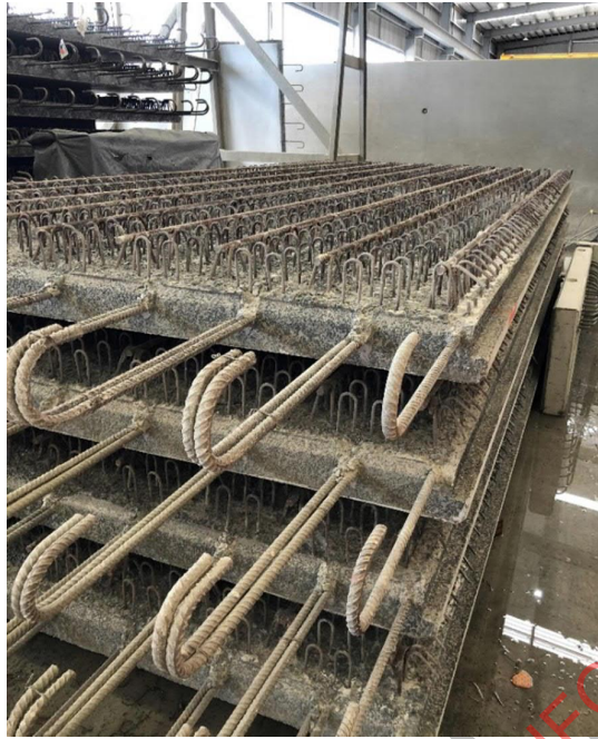
Photo 2: Typical centre precast deck panels
