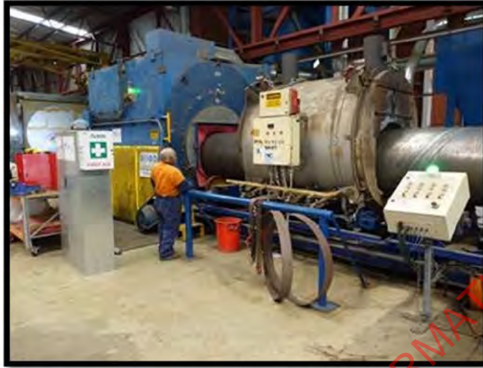
Photo Above: 900mm diameter bulk water pipe being fabricated for Bridge 19
